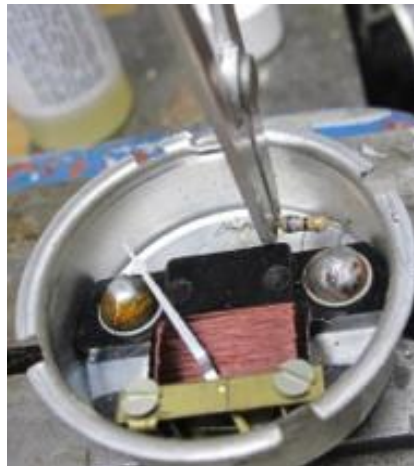
Photo #20 Solder wire using a heat sink
