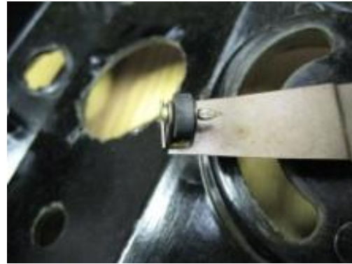
Photo #9 Original AC rollers and crimped pins.
