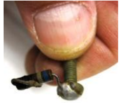
Photo #18 Solder new resistor to screw.
