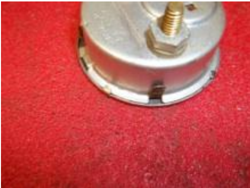
Photo #13 Rotate the back cover Counter Clockwise.
