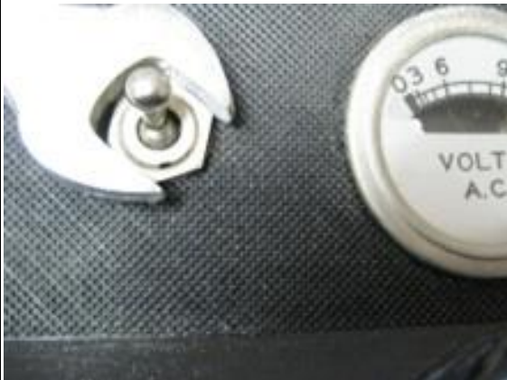
Photo #4 Remove nut holding switch to case.
