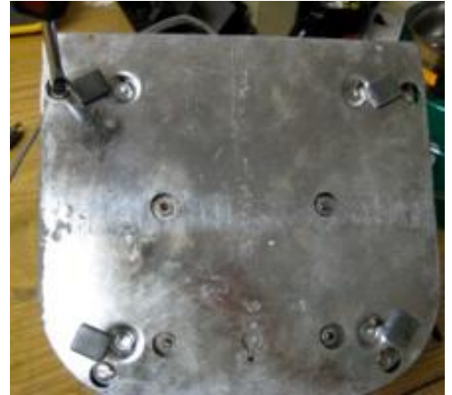
Photo #3 Remove four slot head screws
