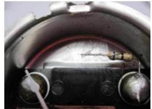
Photo #21 Replacement of resistor complete.
