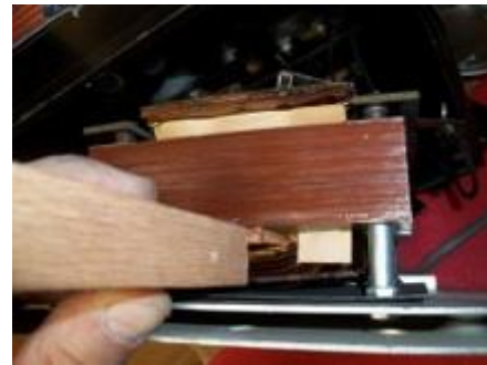
Photo #25 Drive the wood wedge in. The front wedge.
