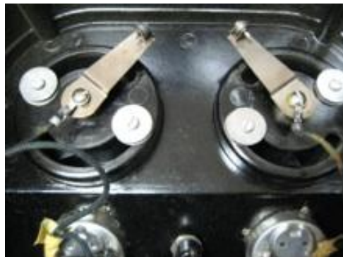
Photo #6 Disconnect wires to throttles
