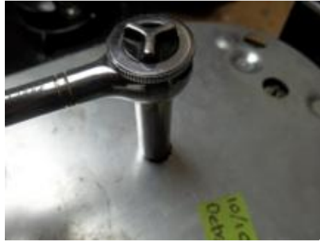
Photo #23 and socket wrench on nuts to tighten core.
