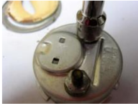
Photo #17 Remove nut holding screw with resistor.
