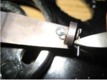
Photo #11 Install new rollers using cotter pins.
