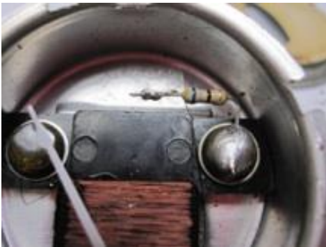
Photo #19 Reinstall nut holding screw and resistor.
