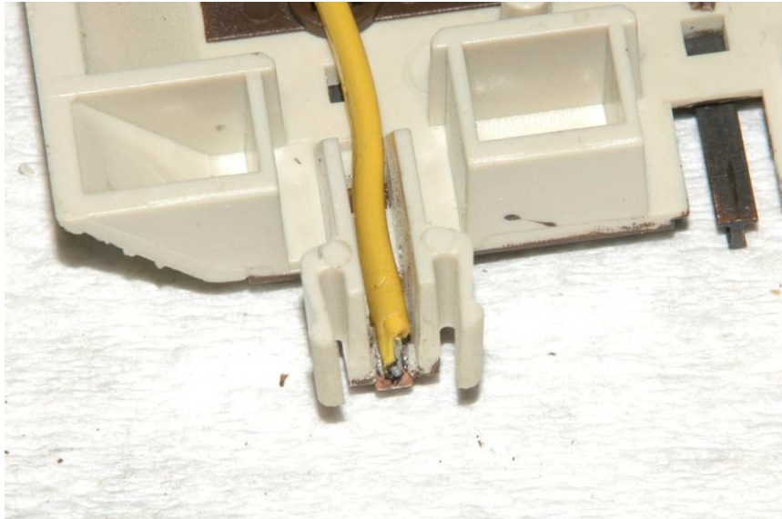
Photo 9 Wire is folded under the track.
