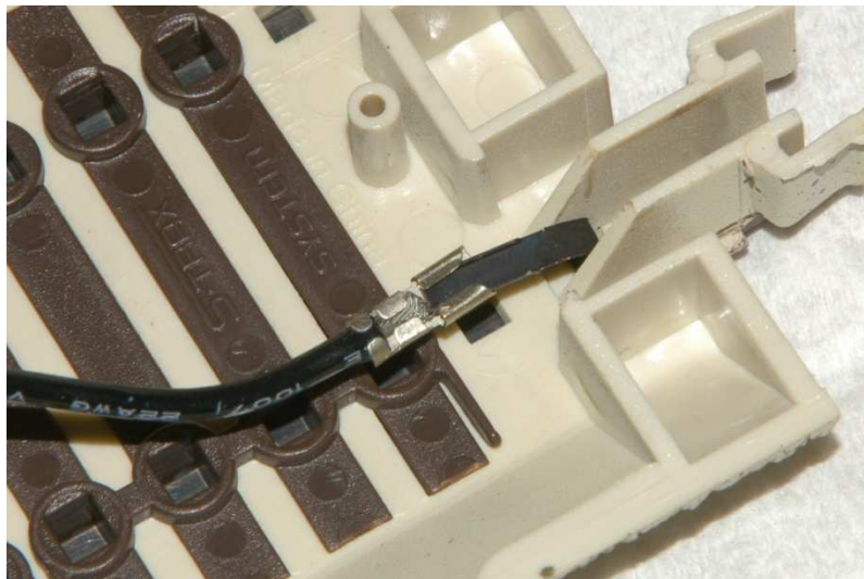
Photo 3 Power wire installed on tab
