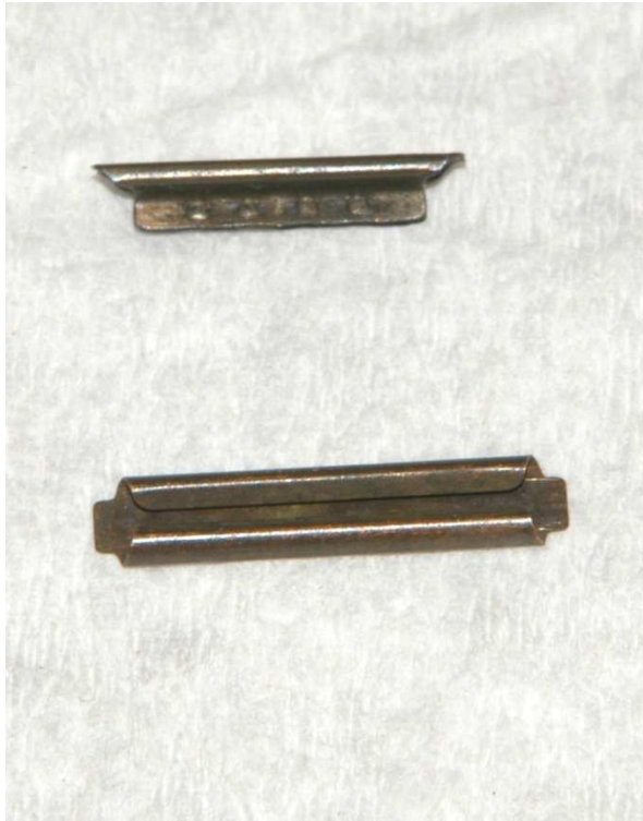
Photo 6 Two types of rail joiners
