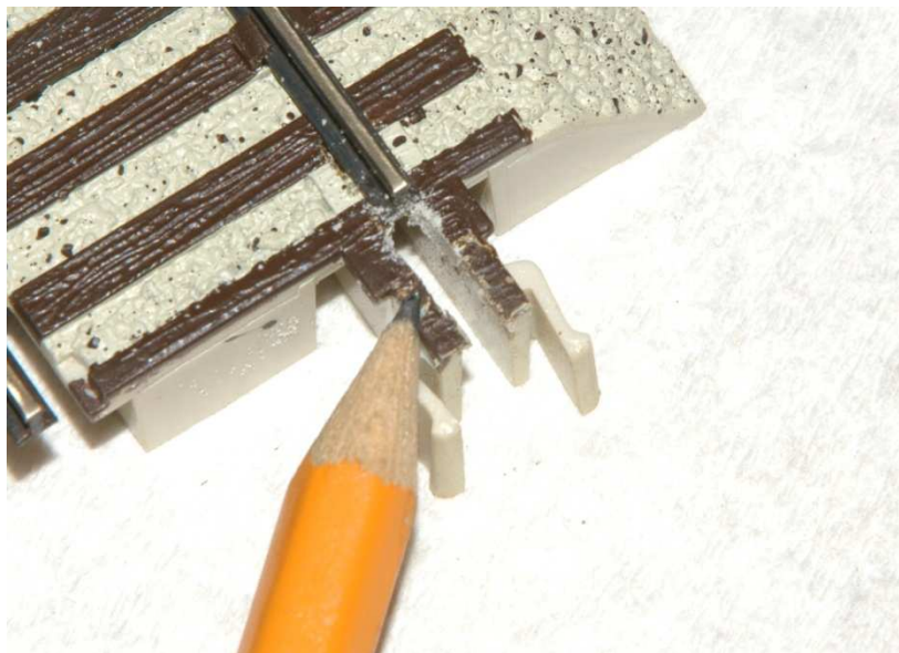
Photo 5 After rail joiner is removed, cut the remaining material back to the edge of the rail.
