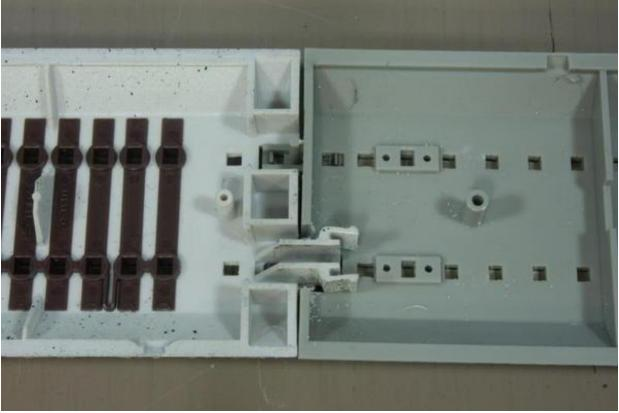
Obviously, the locking feature of these two track systems is gone at this point, but either a metal clip could be formed or a hole could be drilled on the ends for a small screw and nut to hold the track together. For a permanent transition piece, an ABS compatible glue could be used.
