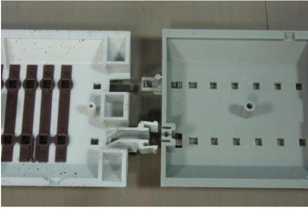
The easiest is to remove the socket on the FasTrack and create an opening for SHS plug to fit. With several cuts with a razor saw and scoring with an X-acto knife, an opening a half inch wide will allow the enough clearance for the SHS plug to pass through, allowing the sections to be joined.
