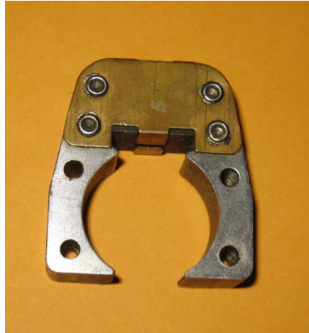
Figure 14: Permanent magnet field for open frame DC motor
