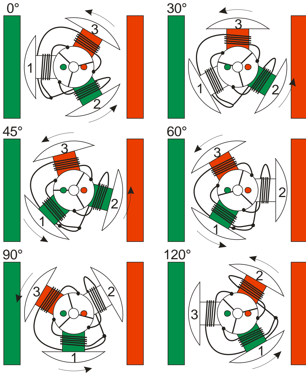
Figure 75: Common Tie-Off Rotor Reverse Direction
