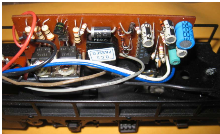
Figure 10: Electronic E-Unit (Lionel American Flyer 6-48005)
