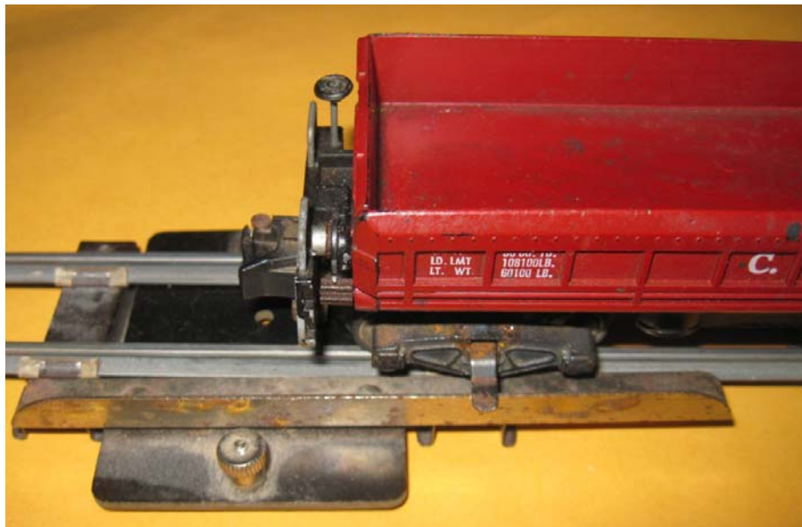
Figure 44: Action car with power contact shoe
