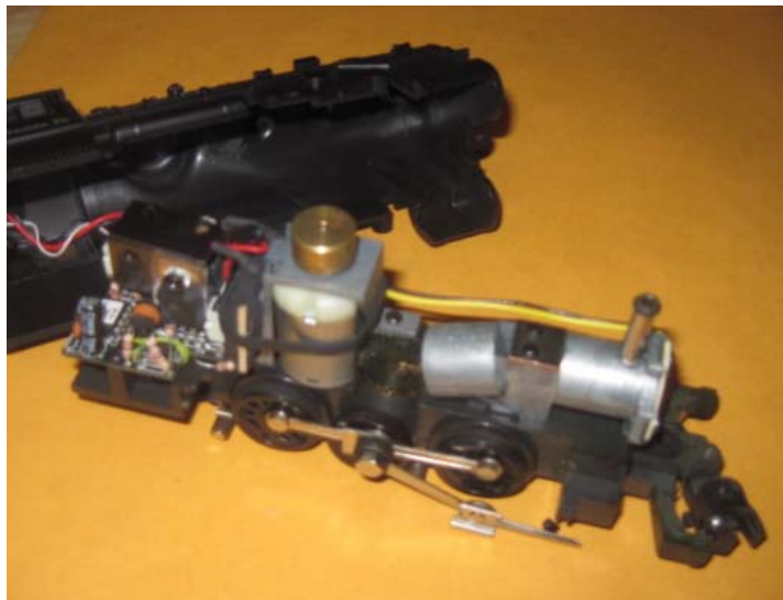
Figure 15: Cam motor (with flywheel) for Lionel American Flyer Docksider
