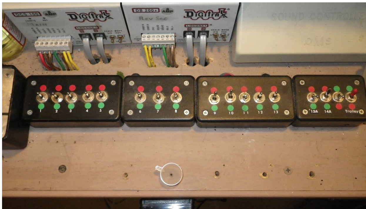
Photo 12: To save control table space, ready boxes can be custom made to save table space. Toggle Switches 8, 9, 10, 11, 13A & 14A are DPDT On-On Latching Switches.
