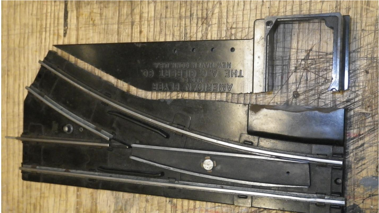
Photo 6: Illustrates the cut line to remove the switch motor tombstone.
