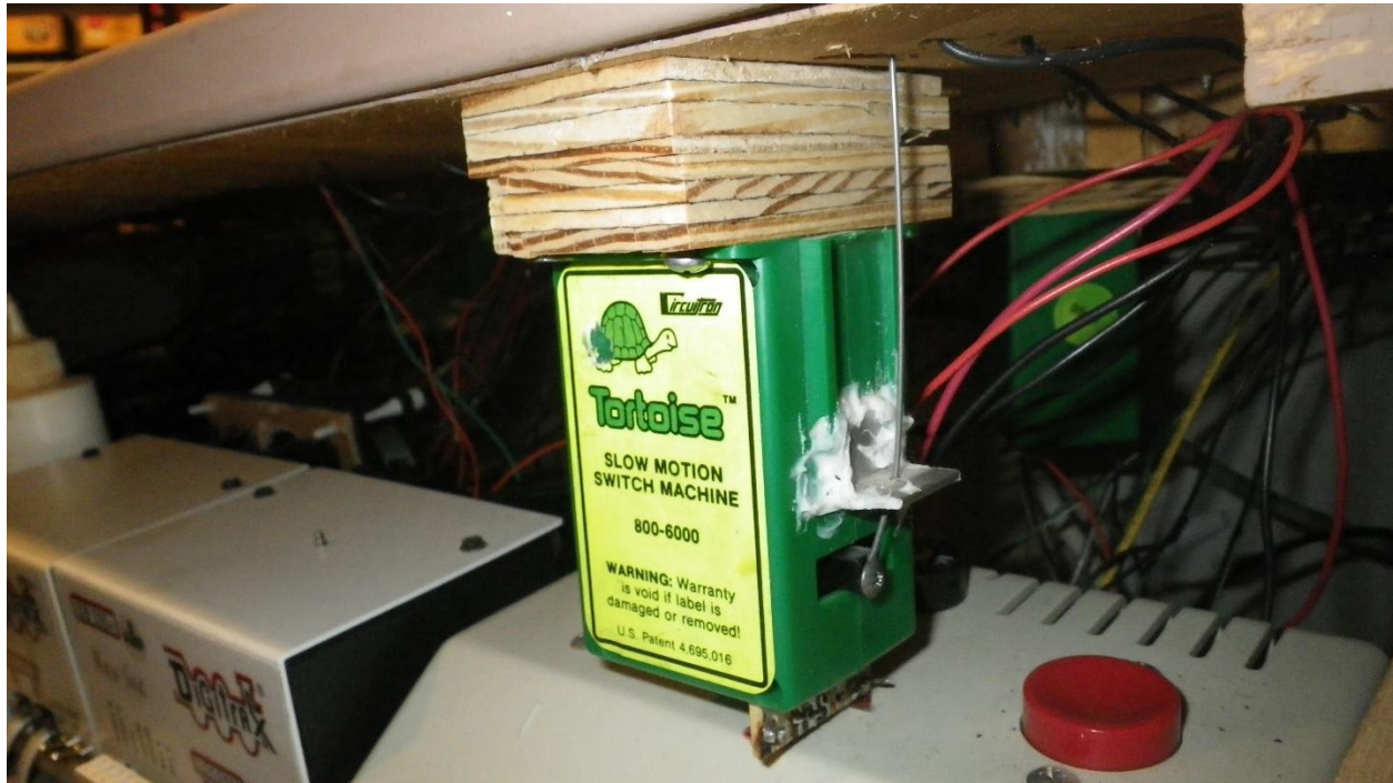
Photo 11: To obtain enough leverage and force, the spring wire has been up-sized, and the adjustable slide bar has been caulked in place. This photo illustrates the additional modifications that are needed to the switch machine.
