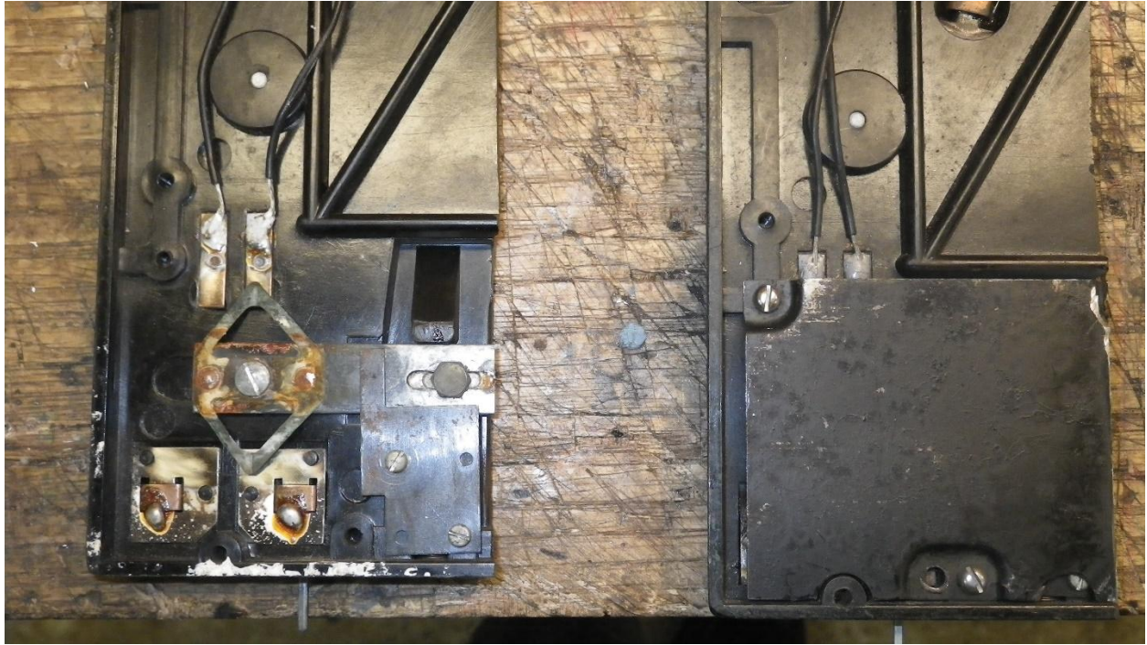
Photo 8: The left image “Flips” the detent cover with new screw holds. The right image shows the detent and slide bar with the “Finished” look.
