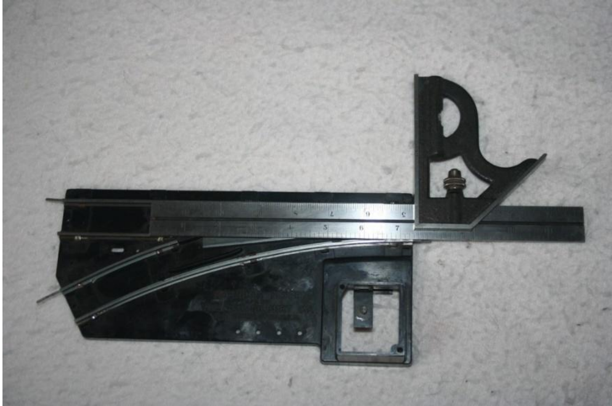
Photo 16: Another key to a compact yard ladder is to cut the straight section of the normal 10" straight track to 7-3/8".
