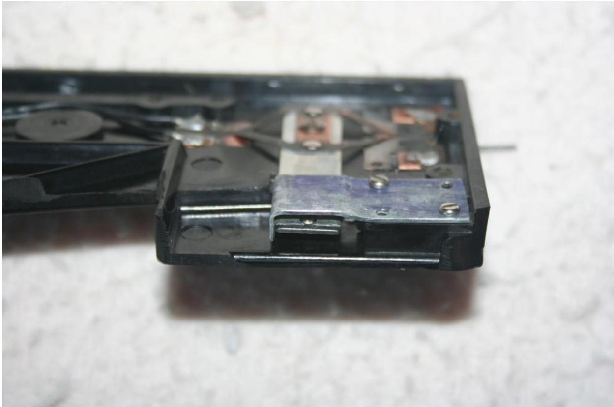
Photo 24: Some AF Switches will need a custom-made combination detent cover and slide bar retainer clip.
