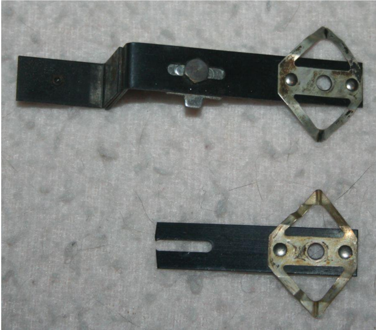
Photo 22: Modification of the slide bar. The image illustrates the detent.
