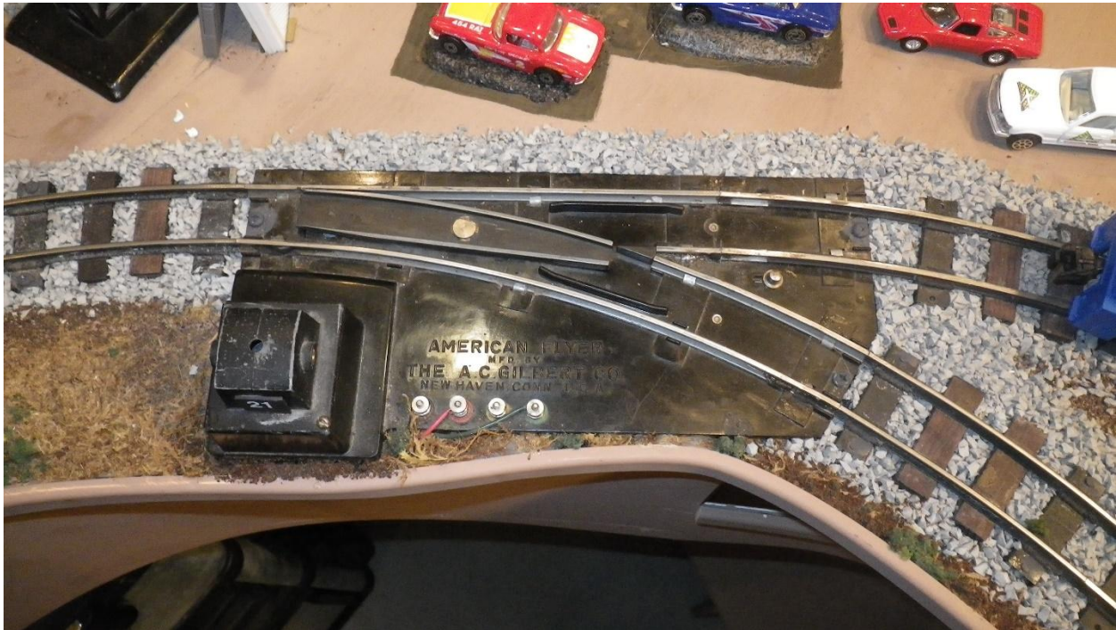
Photo 30: This image illustrates a standard AF Switch with a modification to the straight section of the switch. The curve section is “Started” sooner thus saving space.
