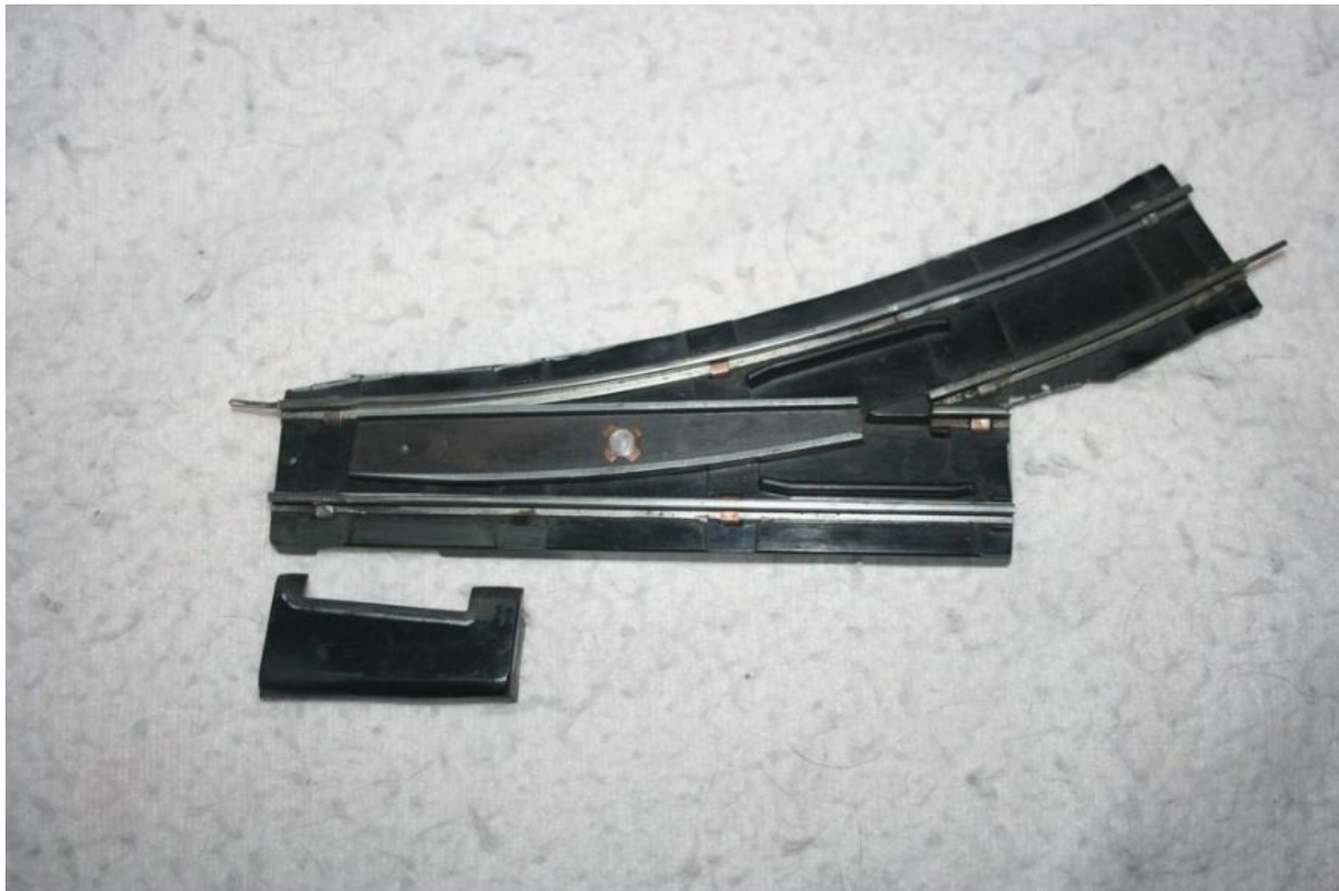
Photo 15: Normal location of the detent is on the inside of the curve section of the switch. By “Flipping” the detent to slide to the outside of the switch, one can compress the yard ladder.
